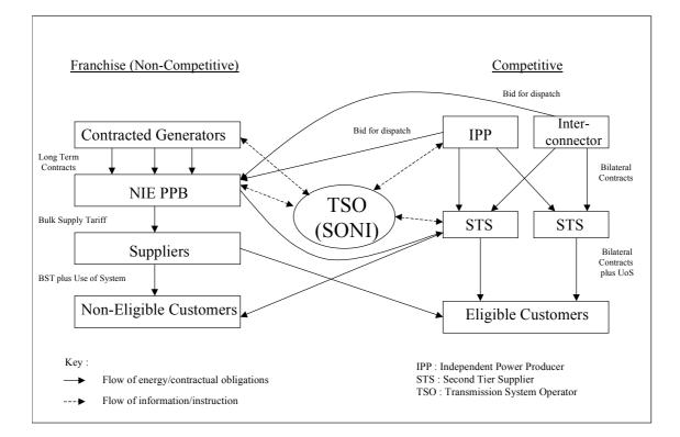
The diagram above shows the effective separation of the two generation markets. Ofreg proposes that the wholesale market of IPPs and interconnectors be merged with the energy produced by generators under long term contract to PPB.
