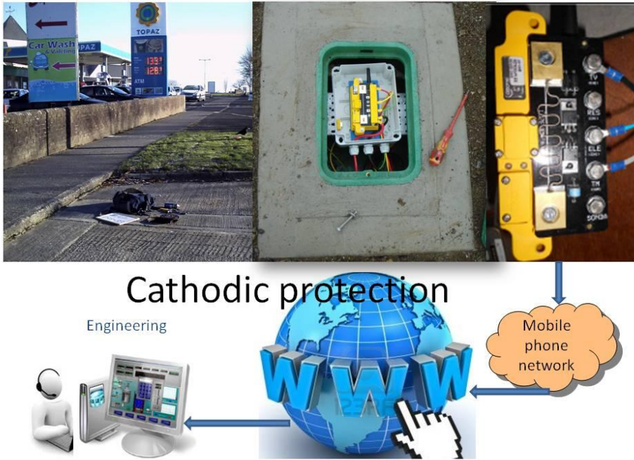
Figure 27 CP Remote Monitoring Architecture
