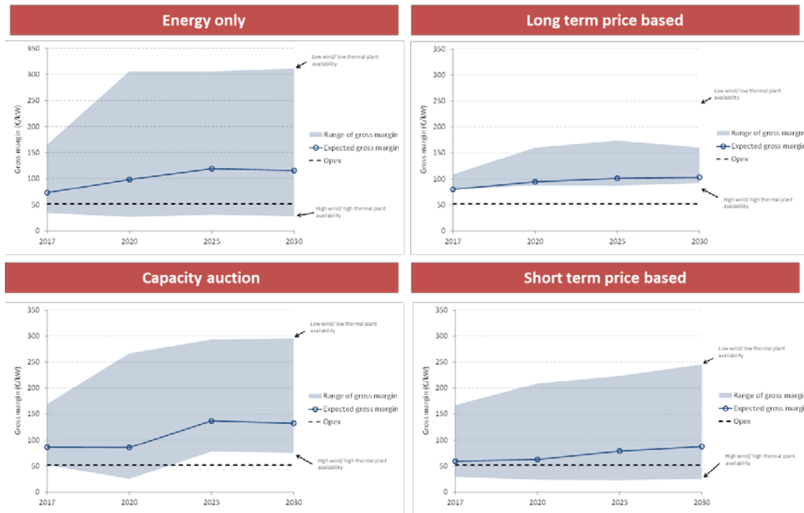
Figure 18 –Gross margin 42 for a 51% efficient (HHV) CCGT under the energy-only market and different types of CRMs (Base Case A)
